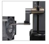
**Diameter Measurements** Simultaneous display of diameter and centerline
