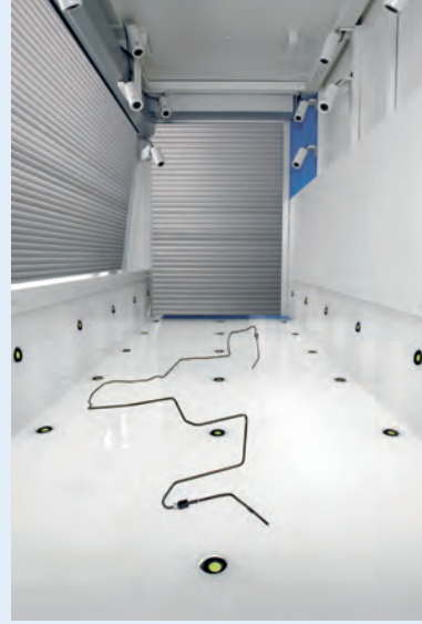
Long and thin tubes can also be measured without fixtures.
