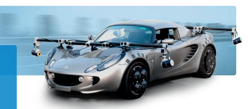
Both systems compute all six degrees of freedom of the wheel and engine motions as absolute values in the vehicle coordinate system. The results can be exported for evaluation through an interface to other software applications (e.g. for motion visualization in CAD).
