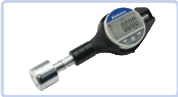
SmartPlug with ceramic contacts
