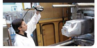
With the MaxSHOT 3D camera, all you have to do is simply place a few coded targets either on the object to be measured or in its environment, take several blocks of convergent photos and launch the bundle adjustment process (image triangulation). Through this process, the reflectors placed on the object can be easily rebuilt in 3D, and the scale bars provided in the measurement volume allow for model scaling.
