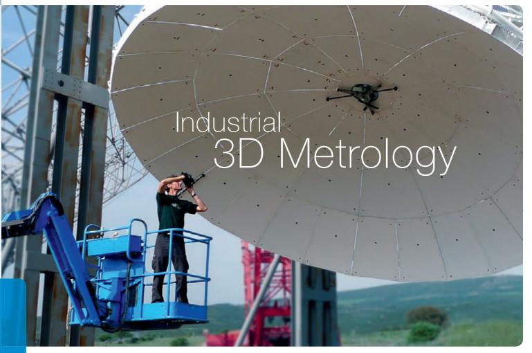
Measurement of a satellite antenna with DPA (photo: sigma3d GmbH)
