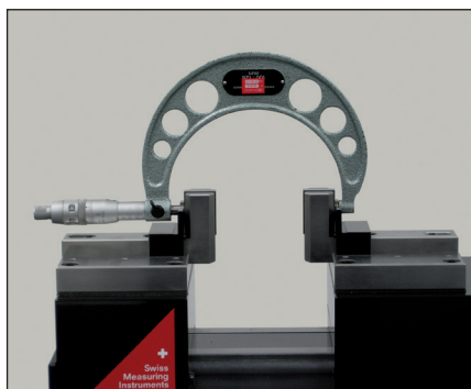
Checking of external micrometers (TEL5/TEL11)
