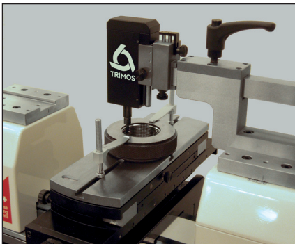
Calibration of thread ring gauges (TA-SU-313/LABC-70/TA-SU-354)
