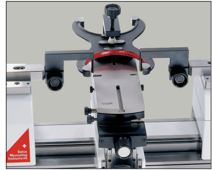
Checking of snap gauges (TA-SU-313/TEL14N)
