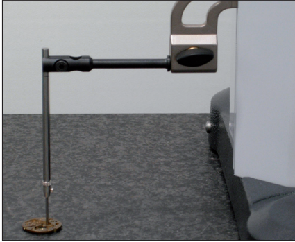
Height measurement of a small board (TA-IH-109/V-50.5/TA-MI-118)
