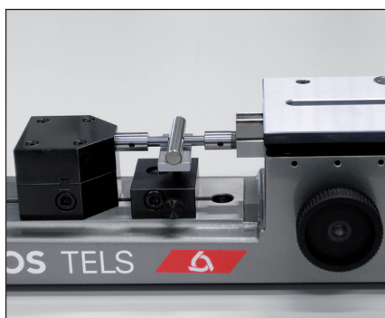
Checking of external diameters (TELS50, TELS5, TELS5.1)
