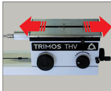
Floating table for more accurate internal measurements
