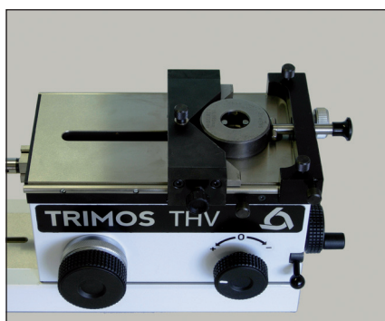
Calibration of plain rings gauges (THV-260)
