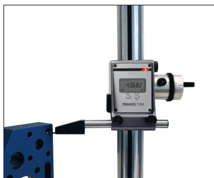
Diameter measurements (TVM4)
